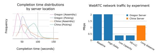
Figure 6: **System Stress Test**: Left: Comparison of completion time distributions between servers located in Oregon vs. in China, when tested from California. Right: Comparison of average throughput of video stream by network experiment, as well as for cross-pacific experiments.
