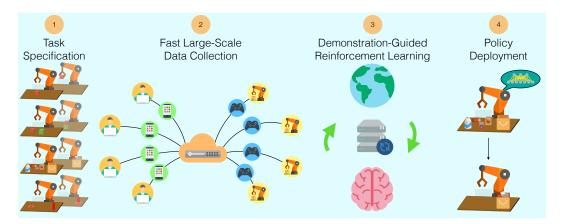
Figure 1: **System overview of ROBOTURK.** ROBOTURK enables quick imitation guided skill learning. Our system consists of the following major steps: 1) specifying a task, 2) collecting a large set of task demonstrations using ROBOTURK, 3) using demonstration-augmented reinforcement learning to learn a policy, and 4) deploying the learned skill in the domain of interest.
