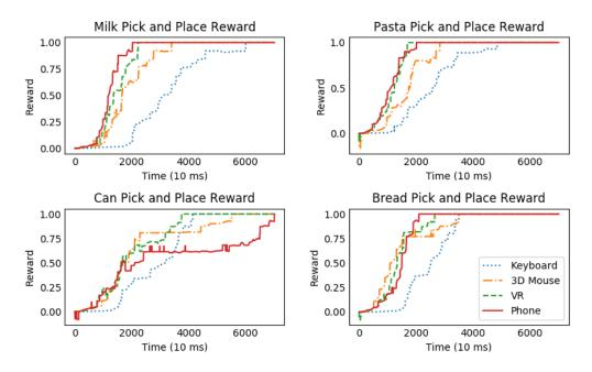
Figure 9: Comparison of environment rewards, which measure the completion of the pick and place operation.
