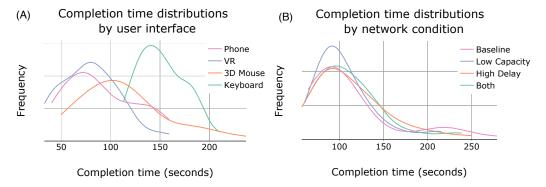
Figure 5: **System Analysis**: **(A)** Comparison of completion time distributions of different user interfaces on the *picking* task. **(B)** Comparison of completion time distributions of different network conditions using the phone interface for the *picking* task.
